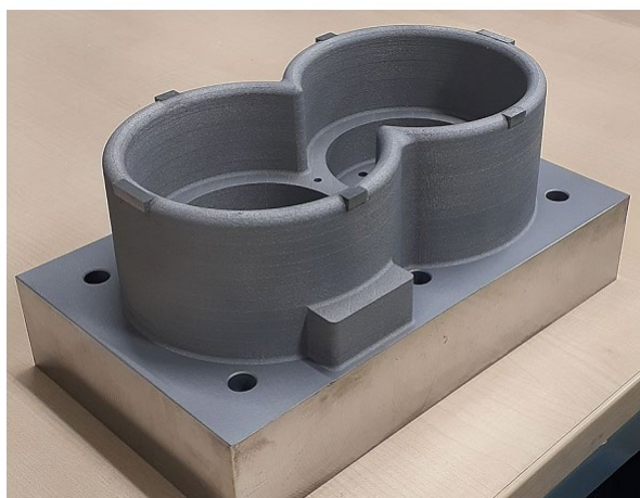
Fig. SVM printed product (221 mm x 146 mm x 67 mm)
